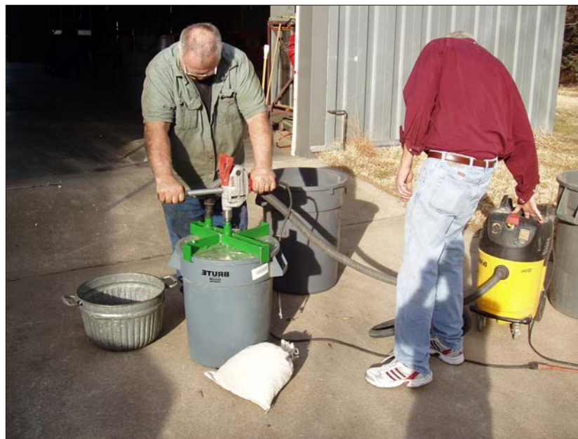
Clockwise from top left: Milkweed seed separator constructed by the USDA-NRCS Plant Materials Center in Manhattan, Kansas. USDA-NRCS staff operating a milkweed seed separator at the Manhattan, Kansas Plant Materials Center. (Photos: USDA-NRCS Manhattan Plant Materials Center.)
